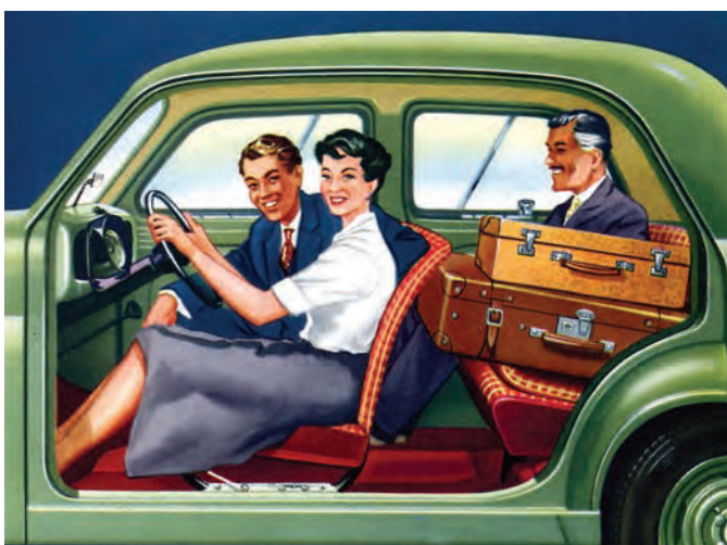
The early Standard Eight had no opening bootlid, but with the rear backrest folded down, carrying capacity was ample.
