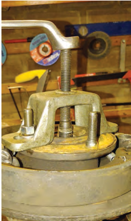
9. Using a hub puller to push the shaft out.
