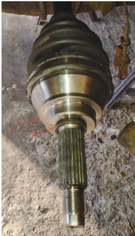
14. Distance piece in place on the new shaft.
