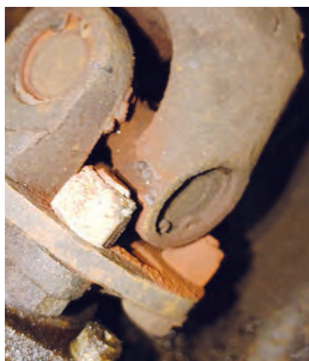
4. Undo the bolts and release UJ flanges from the diff.
