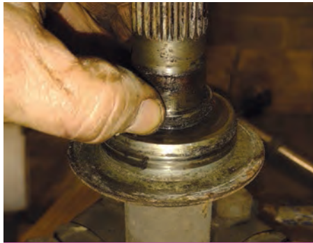
11. Remove the distance piece and shims(s) from the old drive shaft.
