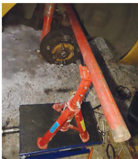
3. Using the spring lifting tool.
