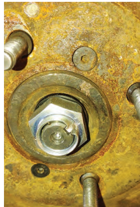
17. The flange on the axle nut deformed into the shaft slot to lock it into place.
