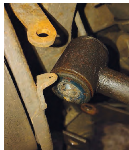
5. Release the tie rod from the vertical link.
