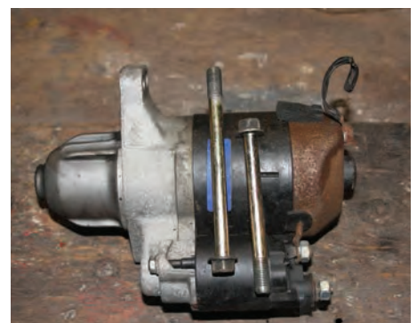
After more than 40 years of use, the bolts holding the starters on were still nicely plated and without rust.
