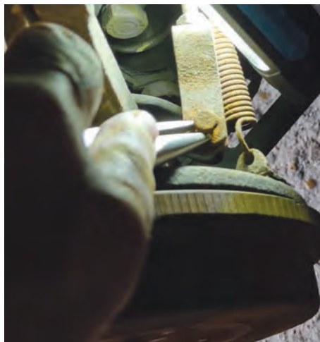
1. Disconnecting the handbrake cable.
