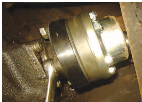
13. Attaching the inner CV joint to the diff flange
